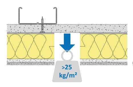
Detail drawing adhesive tensile strength
