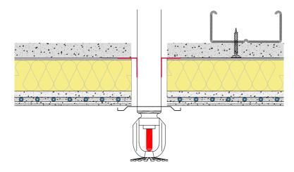
D\_074 Not permeable to air through vapour barrier adhesive tape (red)
